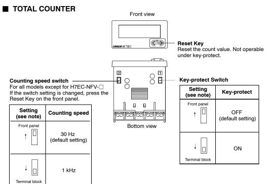
Note: Perform switch setting before mounting to a control panel.
